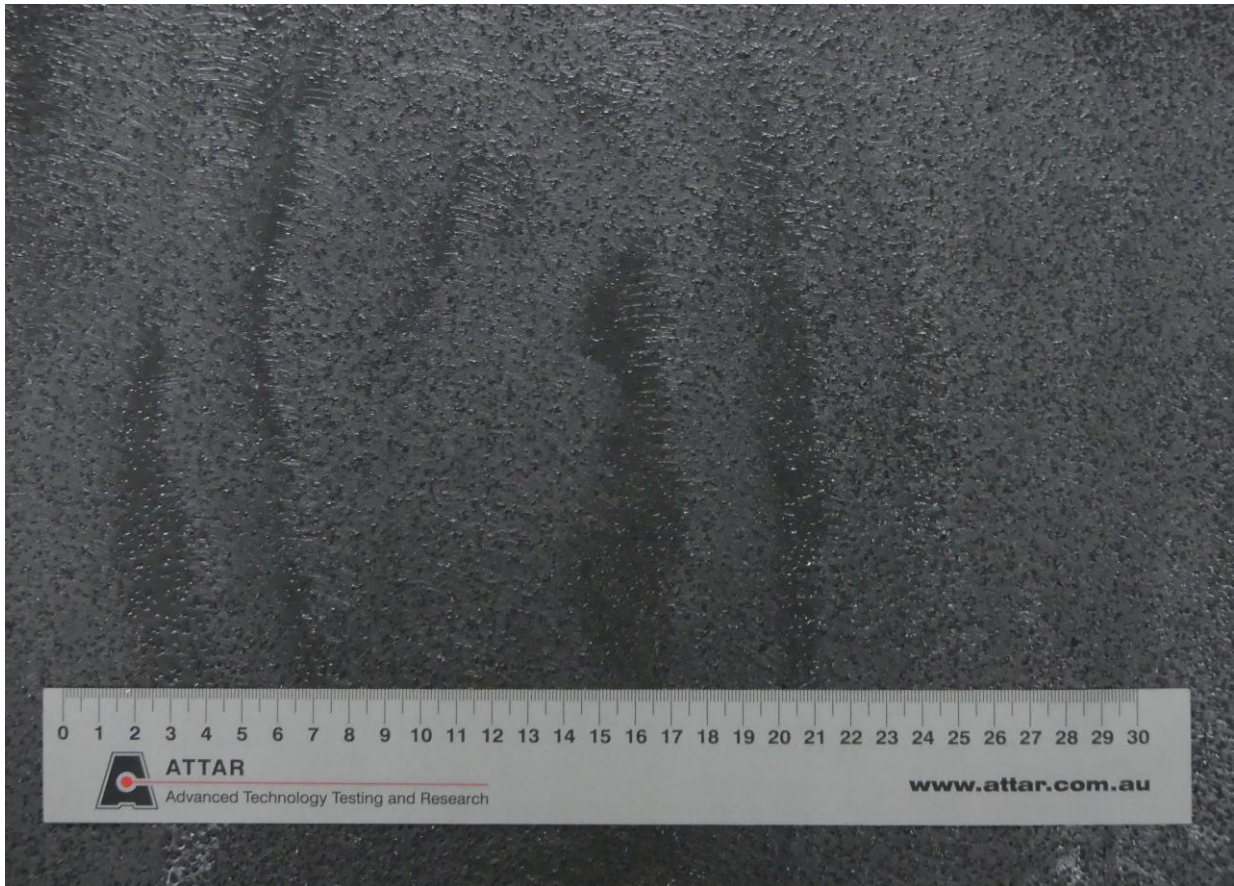
Figure 1: Dulux Avista Tintable Base Sealer with Crushed Glass applied to steel trowel finish concrete
