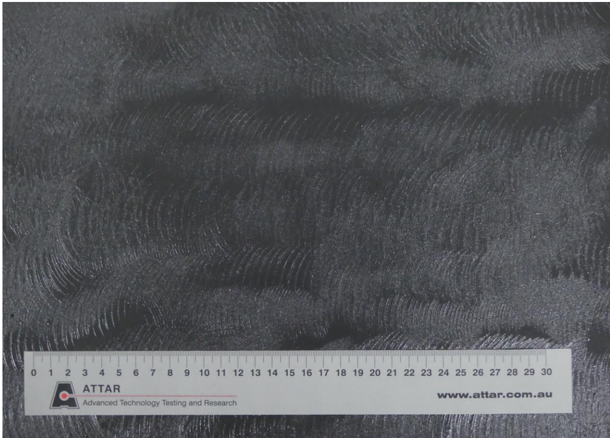
Figure 1: Dulux Avista Tintable Base Sealer applied to steel trowel finish concrete
