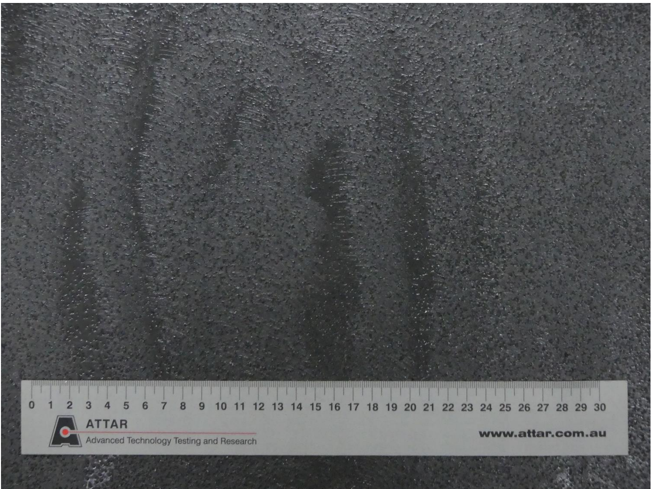
Figure 1: Dulux Avista Tintable Base Sealer with Crushed Glass applied to steel trowel finish concrete.
