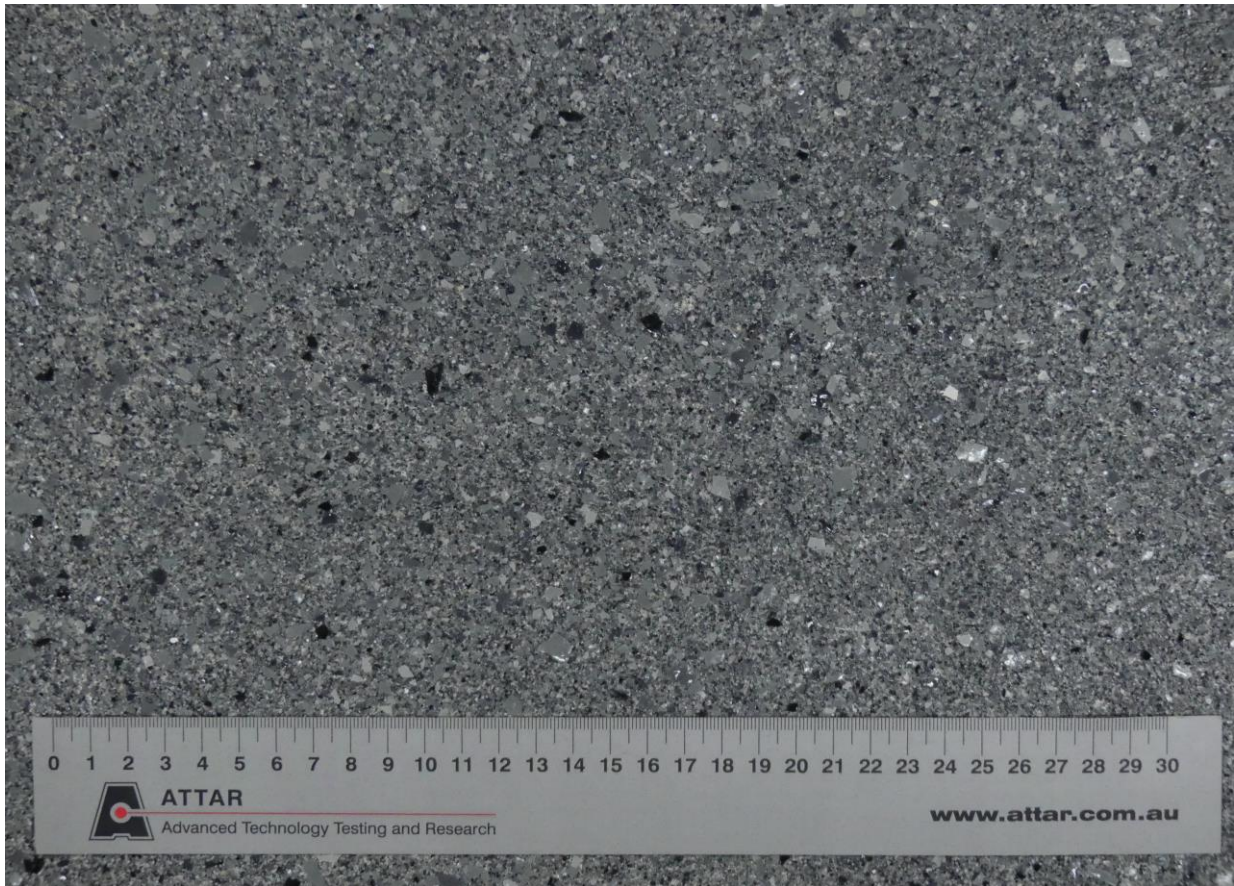
Figure 1: Dulux Avista 2 Pack Urethane Sealer applied to Natural Stone Look Flakes
